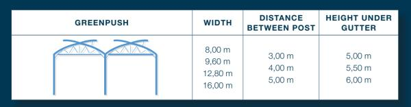
The design of the **GreenPush** plastic mutispan greenhouse makes it possible to consider larger widths. And the same is true for the heights under gutter and under peak. These dimensions allow to imagine new cultivation methods, and new production types.
